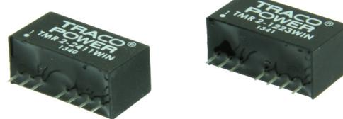
The TMR-2WIN series is a family of isolated 2 W DC/DC converter modules with accurately regulated output voltages and ultra-wide 4:1 input voltage ranges. They require no minimum load and are protected against overload and short circuit.
