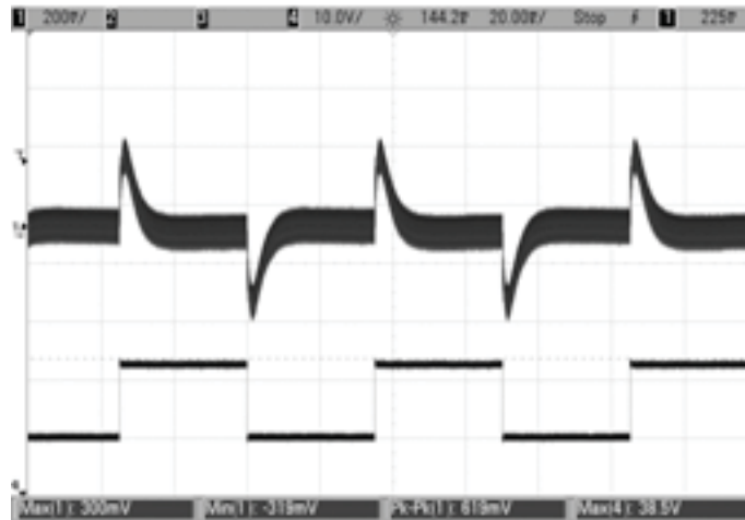
Step Load Transient Response (Vin=48V, Vout=nom, Cload=470µF, Iout=50-75-50% of full load, Ta=+25°C)
